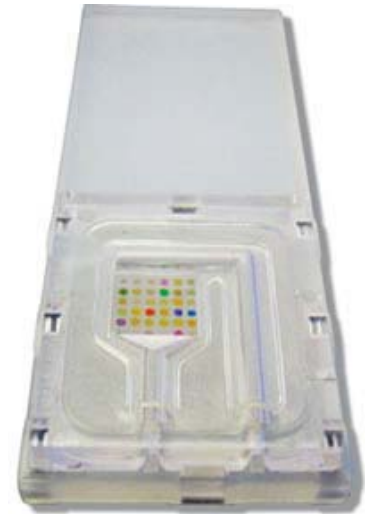
NOSE ON A CHIP: The iSense chemical sensor, developed by Rhodes (below left) and Suslick (below right), mimics nature's design.
