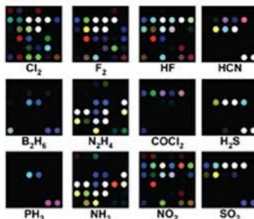
The device boasts more refined detection capabilities than previous efforts, which have relied on more low-strength chemical interactions. The dyes used, the researchers report, are able to respond to a wide catalogue of common, harmful chemicals and register even before toxins exceed permissible exposure limits (PELs).
