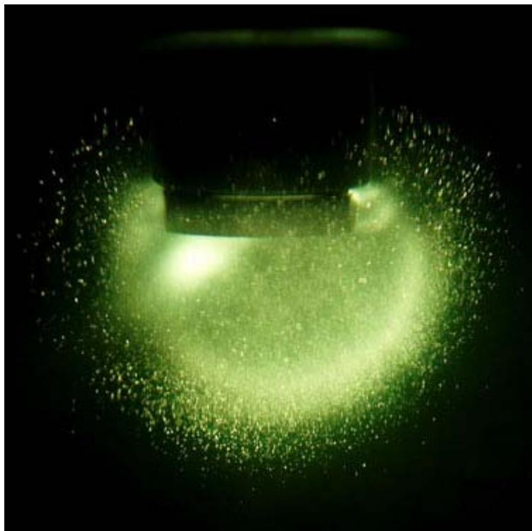
**The big squeeze.** A cloud of bubbles collapsing near a high intensity ultrasonic horn immersed in sulfuric acid
