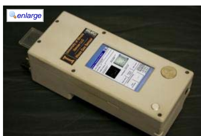
The handheld reader analyzes the color changes in the sensor array to quickly monitor the environment for explosive chemicals. (Credit: Photo courtesy of Ken Suslick)
