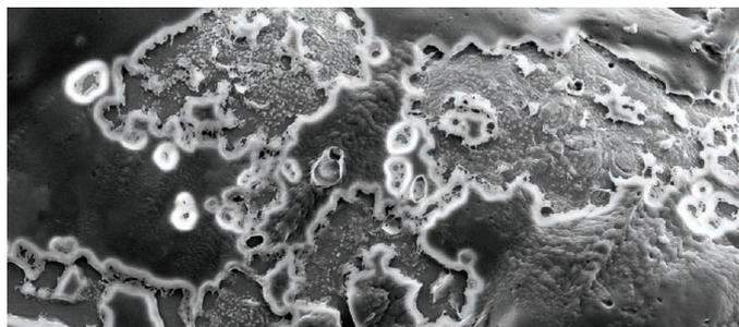
PTFE coating on an NaCl crystal degraded by ultrasonic heating
