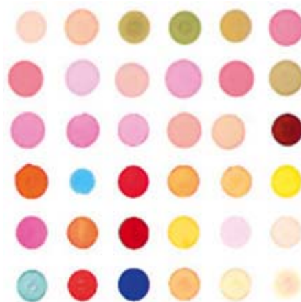
The basis of Suslick's artificial nose is a 1-square-inch array of 36 dyes that change color in predictable ways depending on the chemicals and odorants that are present.
