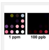
The detector uses a printed array, smaller than a postage stamp, of pigments that change color in the presence of TATP. | Photo courtesy Ken Suslick
