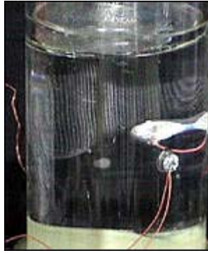
Taleyarkhan's work was done with an acetone liquid in which the normal hydrogen atoms had been replaced with deuterium
