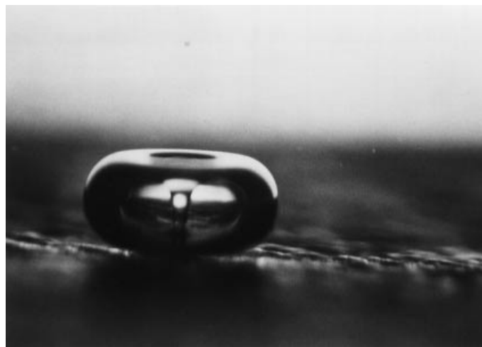
Figure 4. Photograph of liquid jet produced during collapse of a cavitation bubble near a solid surface. The width of the bubble is about 1 mm. Reproduced with permission (13).
