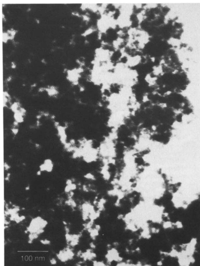
Figure 3 Transmission electron micrograph of amorphous iron powder before crystallization (Philips EM 400T)
