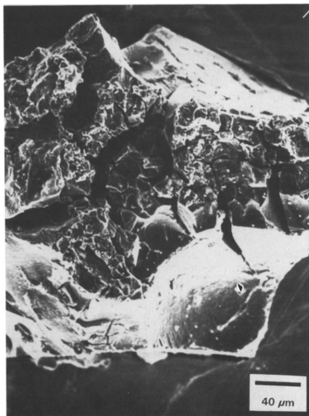
Figure 1 Low resolution scanning electron micrograph of amorphous iron powder produced from ultrasonic irradiation of \text{Fe}(\text{CO})_5 (Hitachi S800)
