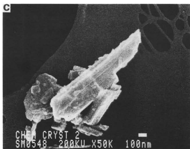
Figure 2 Scanning electron micrographs of \text{MoO}_3 : (a) before ultrasonic irradiation; (b) after 30 min of irradiation; and (c) after 120 min of irradiation. Note changes in scale.
