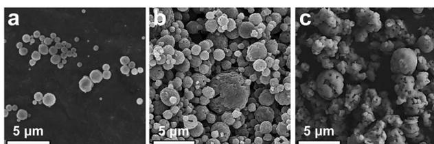
**Fig. 4** High magnification SEM images of the sorbent with Al/Ca = 0.16. (a) before cycling (b) after 2 cycles of calcination/carbonation. (c) after 15 cycles of calcination/carbonation.
