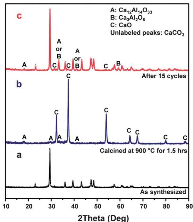
**Fig. 1** XRD patterns of the sample with Al/Ca = 0.16; (a) immediately after collection from the USP setup, (b) after calcination at 900 °C for 1.5 h and (c) after 15 cycles of calcination/carbonation. The XRD peak labels given for CaCO<sub>3</sub>, Ca<sub>12</sub>Al<sub>14</sub>O<sub>33</sub>, Ca<sub>3</sub>Al<sub>2</sub>O<sub>6</sub> and CaO are from ICDD PDF cards 04-007-8659, 00-009-0413, 04-008-8069 and 04-005-4757 respectively.
