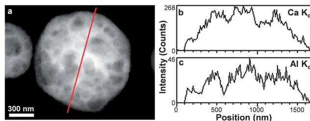
**Fig. 2** (a) STEM image and EDX line scan analysis of a particle with Al/Ca 0.16; (b) Ca K<sub>α</sub> signal with 268 max counts, and (c) Al K<sub>α</sub> signal with 46 max counts. The red line in (a) indicates the line scan analysis path (~1.7 μm, 15 analysis points).
