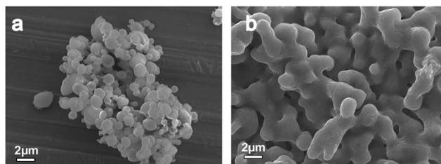
**Fig. 5** SEM images of the hollow pure CaO sorbent. (a) After 2 cycles of calcination/carbonation. (b) After 25 cycles of calcination/carbonation. This picture shows that CaO particles retained their spherical morphology after a few cycles of adsorption/desorption and lost their structure in an increased number of cycles.
