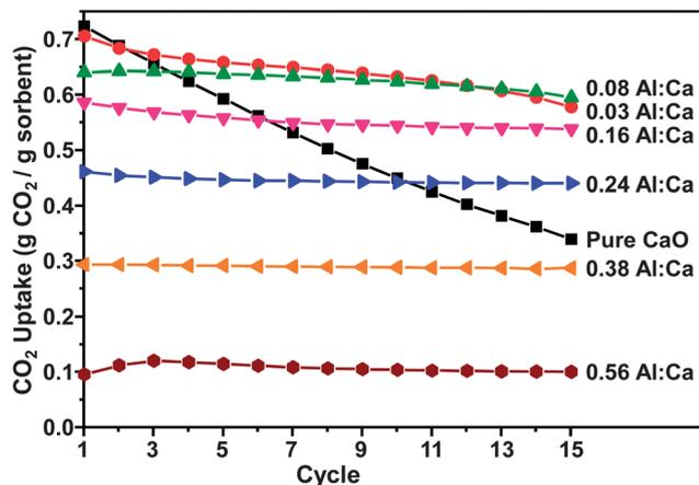
**Fig. 3** CO<sub>2</sub> uptake by Al-containing sorbents during 15 cycles of calcination/carbonation; calcination at 950 °C for 5 min under 100% N<sub>2</sub> and carbonation at 710 °C for 30 min under 100% CO<sub>2</sub>. Incorporating low concentrations of Al<sub>2</sub>O<sub>3</sub> significantly improves the cycling stability over 15 cycles.
