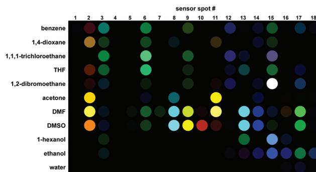
Fig. 1 Difference maps showing the colorimetric sensor array response to eleven analytes at 10% of their saturation vapor pressure after 5 min of exposure (averages of five trials each are shown). A color range of 1.5–8.5 was expanded to 8-bit color range (*i.e.*, 0–255) for visualization. A complete list of the 18 sensor spot formulations can be found in Table S3.†
