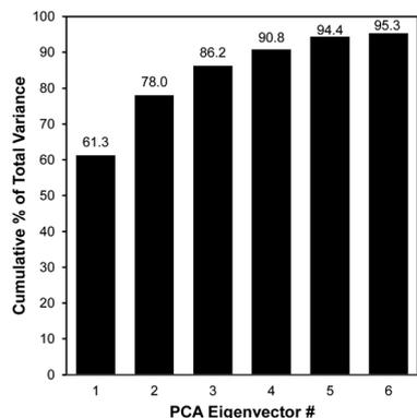
Fig. 3 Scree plot of the principal components from PCA from 11 analytes and a  $N_2$  control. Six dimensions are required to define 95% of the total variance.
