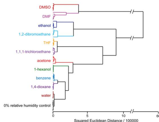
Fig. 2 Hierarchical cluster analysis of the colorimetric array response to 11 common organic solvents and the control. The 11 analytes were run in quintuplicate and the dry  $N_2$  control was run in septuplicate. The HCA used minimum variance (*i.e.*, ward's method) for clustering. No misclassifications were observed among the 62 trials.
