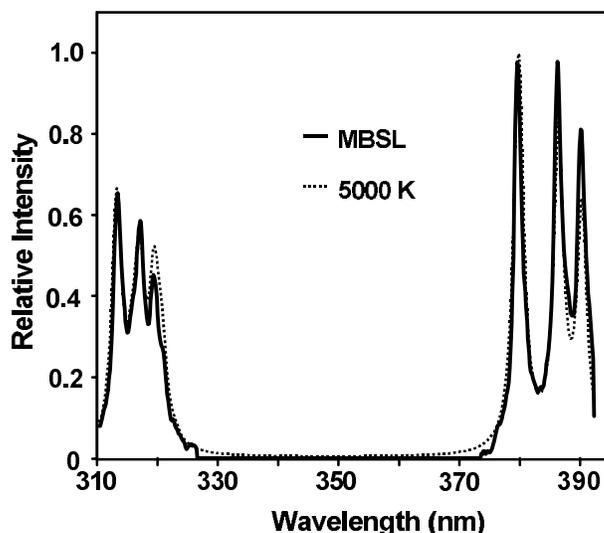
Figure 8. Sonoluminescence of excited-state Mo atoms produced during sonolysis of  $\text{Mo}(\text{CO})_6$  dissolved in silicone oil under Ar. Effective emission temperature is  $4750 \pm 400$  K.
