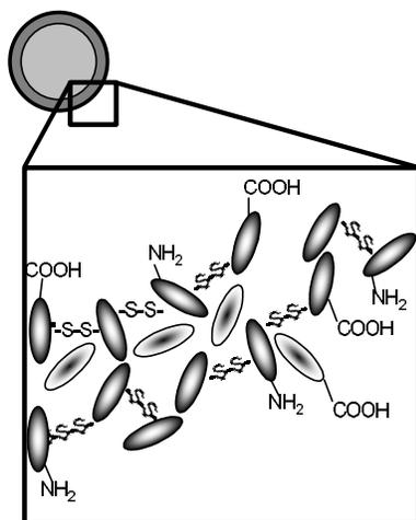
Figure 14. Disulphide cross-linking holds the protein microspheres together.
