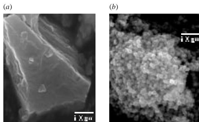
Figure 12. Morphology of (a) conventional and (b) sonochemically prepared MoS<sub>2</sub> (Mdleleni *et al.* 1998).
