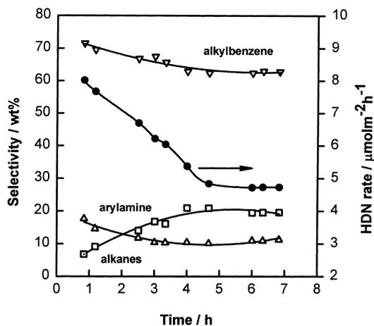
Fig. 3. Variation of reaction rates and selectivity of sonochemically prepared  $\text{Mo}_2\text{C}$  with time on stream for HDN of indole. Indole feeding rate= $0.1 \text{ cm}^3 \text{ h}^{-1}$ ,  $\text{H}_2$  flow rate= $90 \mu\text{mol s}^{-1}$ , catalyst loading= $2 \text{ mmol}$ , temperature= $673 \text{ K}$ .
