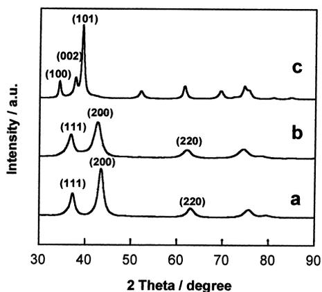
Fig. 4. X-ray diffraction patterns of  $\text{Mo}_2\text{N}$  and  $\text{Mo}_2\text{C}$  after indole HDN at temperatures between  $573$  and  $773 \text{ K}$ : (a)  $\text{Mo}_2\text{N}$  (fcc); (b)  $\text{Mo}_2\text{C}$  (fcc) and (c)  $\text{Mo}_2\text{C}$  (hcp).
