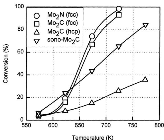
Fig. 1. Catalytic activity as a function of temperature over  $\text{Mo}_2\text{N}$  and  $\text{Mo}_2\text{C}$  in indole HDN. Indole feeding rate= $0.1 \text{ cm}^3 \text{ h}^{-1}$ ,  $\text{H}_2$  flow rate= $90 \mu\text{mol s}^{-1}$ , catalyst loading=2 mmol.
