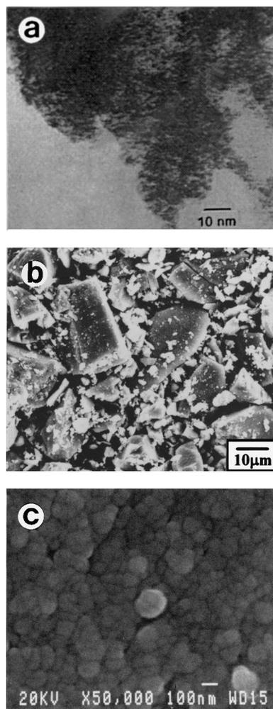
Fig. 7. Transmission electron microscopy showing morphologies of sono-chemically prepared  $\text{Mo}_2\text{C}$  before reaction (a), scanning electron microscopy showing morphology after indole HDN at temperatures between 573 and 773 K, overall morphology (b) and detailed morphology of a platelet (c). The dark backgrounds in (b) and (c) represent graphite stubs that were used to support SEM sample powders.
