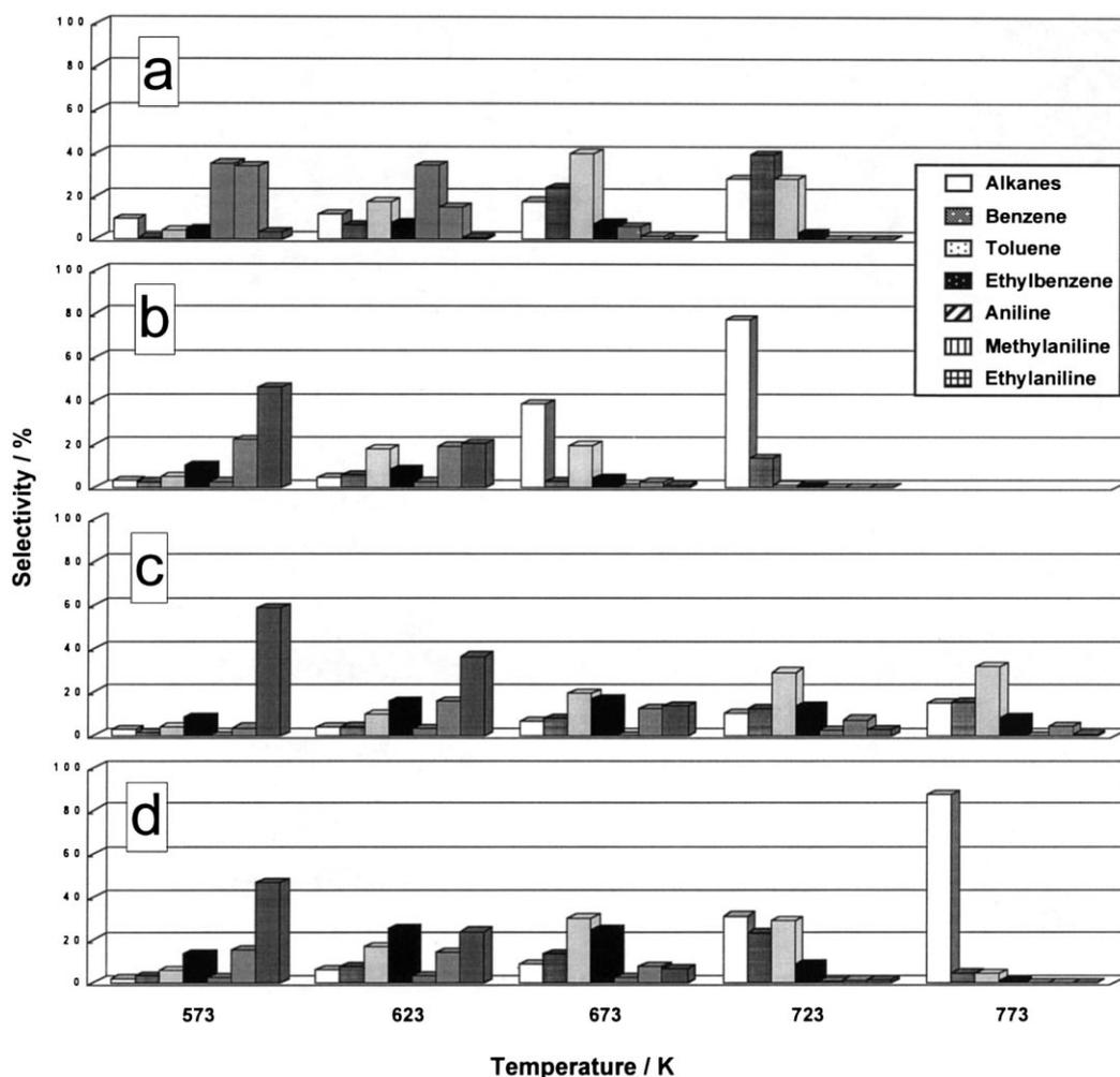
Fig. 2. Product distributions as a function of temperature over  $\text{Mo}_2\text{N}$  and  $\text{Mo}_2\text{C}$  with different structures for HDN of indole: (a)  $\text{Mo}_2\text{N}$  (fcc); (b)  $\text{Mo}_2\text{C}$  (fcc); (c)  $\text{Mo}_2\text{C}$  (hcp) and (d) sono- $\text{Mo}_2\text{C}$ . Indole feeding rate =  $0.1 \text{ cm}^3 \text{ h}^{-1}$ ,  $\text{H}_2$  flow rate =  $90 \mu\text{mol s}^{-1}$ , catalyst loading =  $2 \text{ mmol}$ .
