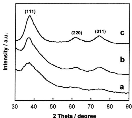
Fig. 6. X-ray diffraction patterns of sonochemically prepared  $\text{Mo}_2\text{C}$  (a) after synthesis, (b) after He treatment at 723 K for 12 h and (c) after indole HDN at temperatures between 573 and 773 K.
