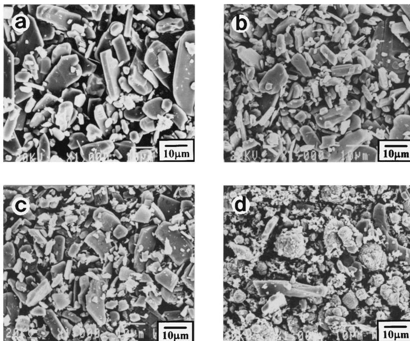
Fig. 5. Scanning electron microscopy showing morphologies of (a)  $\text{MoO}_3$ , (b)  $\text{Mo}_2\text{N}$  (fcc), (c)  $\text{Mo}_2\text{C}$  (fcc) and (d)  $\text{Mo}_2\text{C}$  (hcp) after indole HDN at temperatures between  $573$  and  $773 \text{ K}$ . The dark backgrounds represent graphite stubs that were used to support sample powders.
